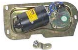
[WIPER MOTOR FOR FLYER (SUZUKI)] [RZ.ZD1331G]
